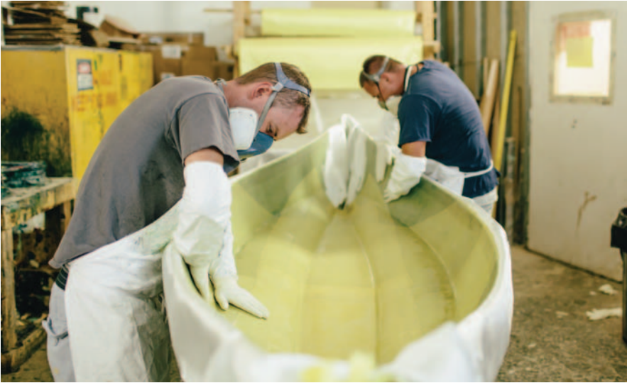
The skin of the Vermont Dory includes layers of Kevlar and fiberglass, which make it strong and light.
